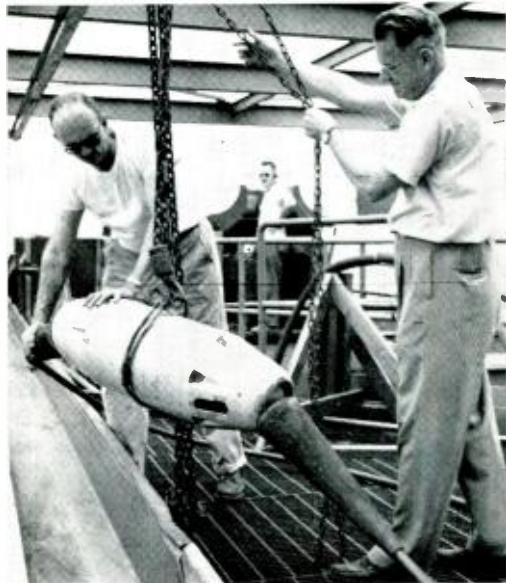
Experimental amplifier about to be “launched” from “cable ship.” Like a giant string of beads, amplifiers and connecting cable must be overboarded without stopping the ship.
