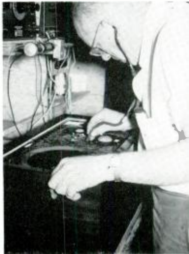
Fig. 4. Stethoscope check for air leaks. The speaker is being driven by a 20-cps signal.
