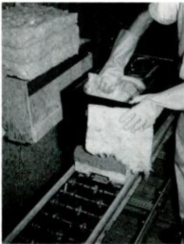
Fig. 2. Fiberglass, in weighed-out amounts, being used to fill an AR speaker cabinet.
