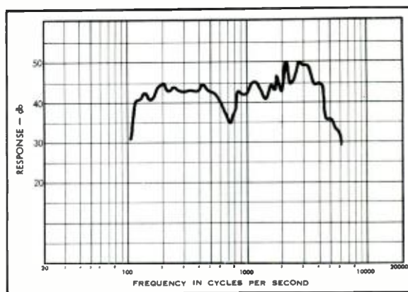
Fig. 4 (left). Response-frequency characteristic of 115-cps cutoff exponential horn. Measured outdoors on horn axis two inches from mouth. Fig. 5 (right). Response-frequency characteristic of 3½-inch piston-diaphragm loudspeaker. Measured 12 feet from diaphragm, in highly absorbing room.
