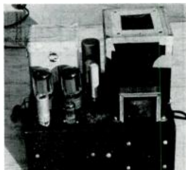
Fig. 5. Another embodiment of the "Universal" amplifier—this one uses silicon rectifiers in the power supply section.
