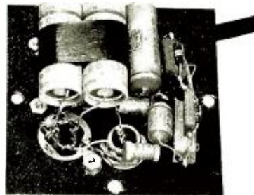
Fig. 8. Under-chassis view of the preamplifier to show details of the input side.
