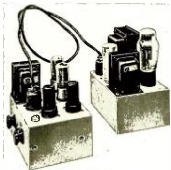
Fig. 1. Separate chassis for the amplifier and power supply simplify mounting in many applications.
