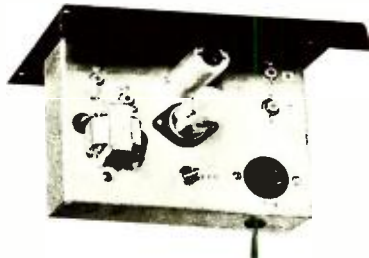
Fig. 3. Detail of the mixer chassis. The input connectors marked "L" and "R" correspond with the left and right gain controls.
