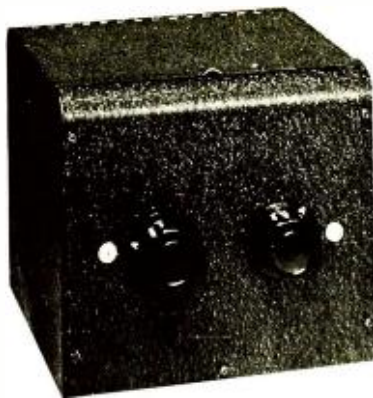
Fig. 1. The simplicity of the front panel of the mixer is made possible by mounting the connectors and switches on the chassis so they are accessible by opening the cabinet top.
