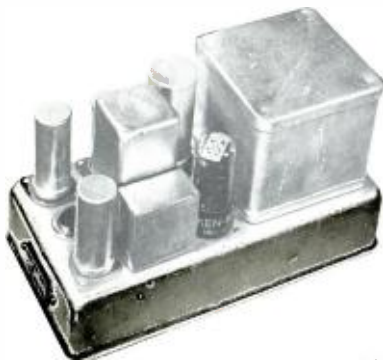
Fig. 14. External view of power supply used in the fixed installation.
