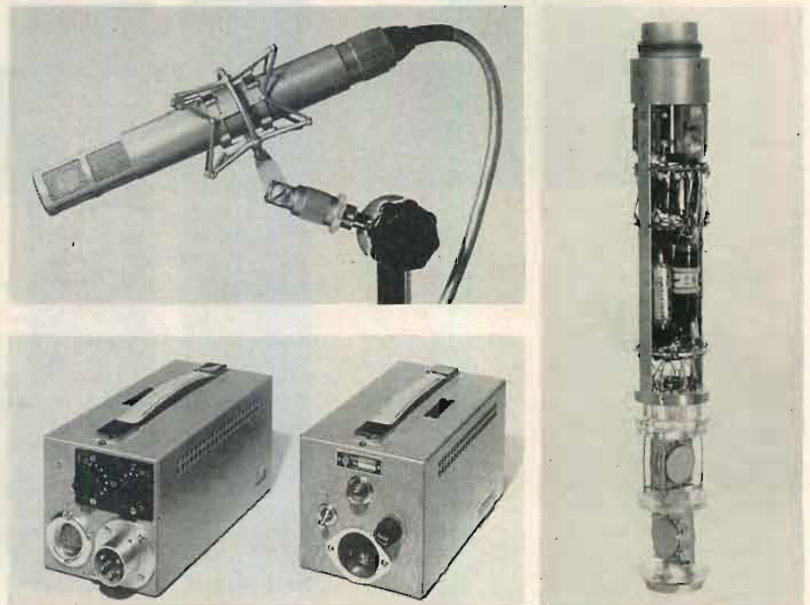
Fig. 11. (A) Internal and (B) external views of Telefunken SM-2 stereo condenser microphone and (C) power supply. (Courtesy Gotham Audio Sales Co. Inc.)
