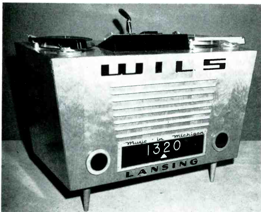
Fig. 1. Front view of the Disc-Hop Consolette. The desk is 24 in. wide, 48 in. long, and 32 in. high.
