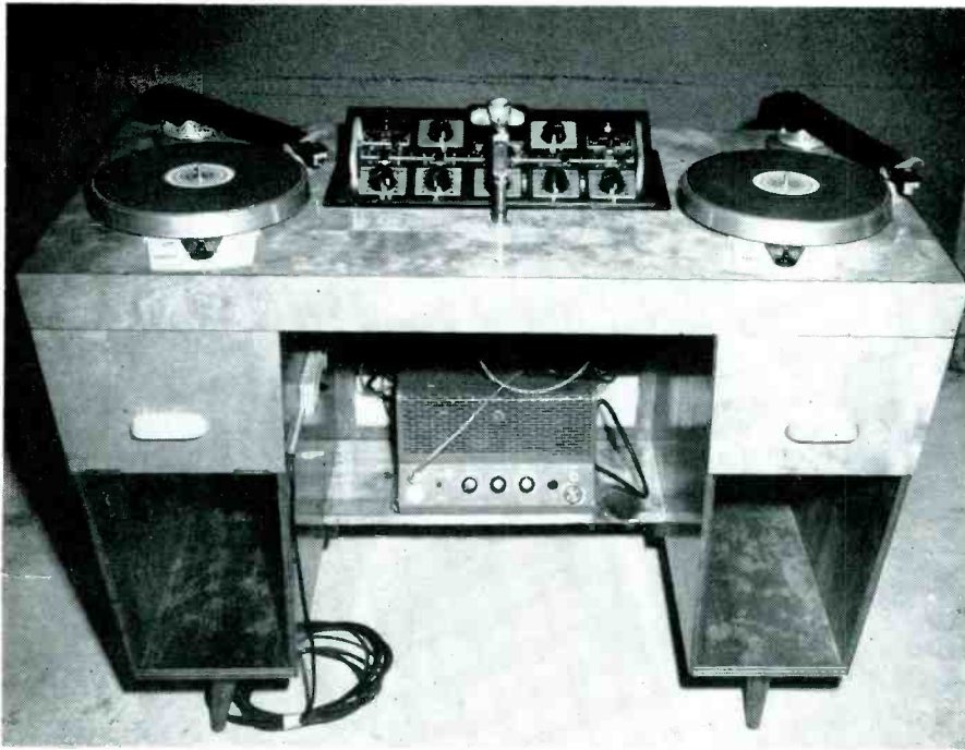
Fig. 2. Back and top view of the desk. Note drawers for parts storage and compartments for records. The p.a. amplifier rests on the shelf between the two pedestals.
