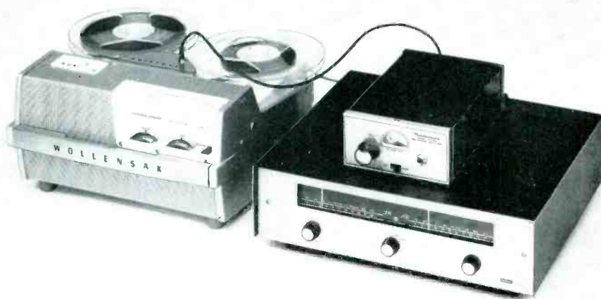
Fig. 1. Stereo recording setup, with AM-FM stereo tuner and additional recording amplifier used with converted Wollensak tape recorder.
