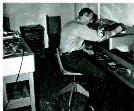
Transcribing machines. A 33 1/3-rpm record is being transferred onto tape.
