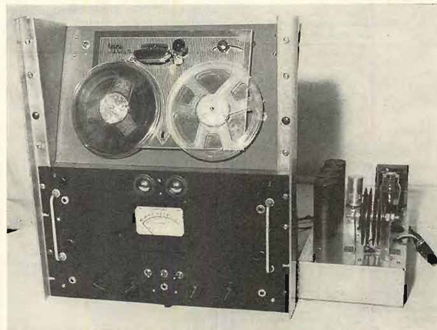
Fig. 6. The tape deck is attached to the amplifier by means of two "Tee" bars. Although the power supply is shown next to the amplifier it should be no closer than three feet when it is being used.
