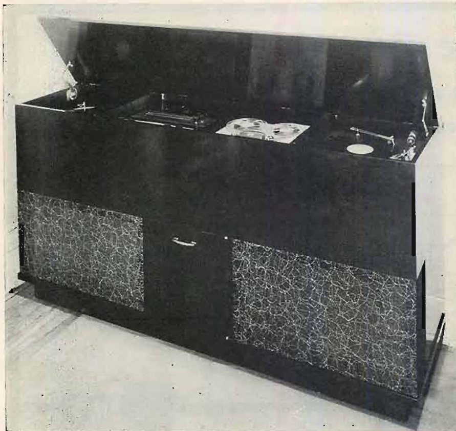
Fig. 3. View of complete console with top up and ready for use. Grille-cloth areas cover two AR-1 speaker systems.
