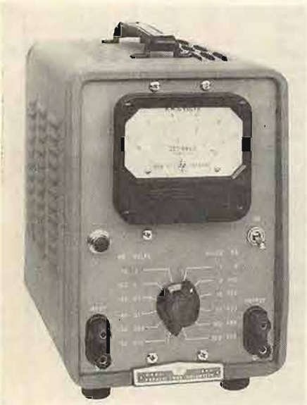
Fig. 6. A typical audio voltmeter. Although the scale is marked "Decibels," the reference level indicated on the meter is given as 1 mw/600 \omega . Observe that 0 on the db scale is directly under 0.775 volts on the rms voltage scale. The meter is in reality a dbm meter. (Courtesy Hewlett-Parkard Co.)
