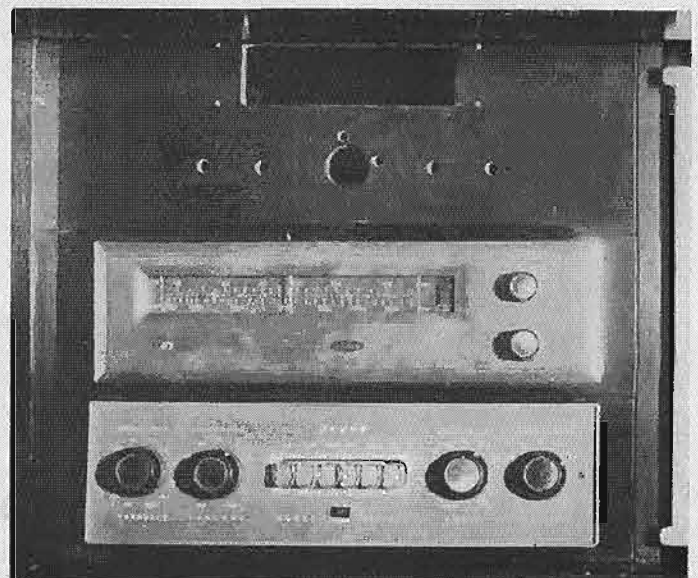
Fig. 6. Tuner and preamp panels are mounted on individually replaceable mounting boards. Pre-cut panel is for TV tuner.
