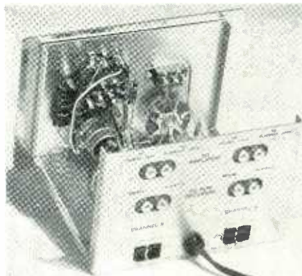
Fig. 4. Rear and inside view of Scott Stereo-Daptor. Both audio and power circuits are controlled.
