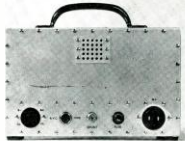
Fig. 11. Rear of case, showing ventilating grille and decal markings.
