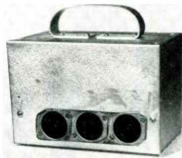
Fig. 5. Rear view of unit. Entire chassis may be taken out of the case by removing two round-head screws. Hubbell twistlock connectors—for microphones—are flush with surface of cabinet.
