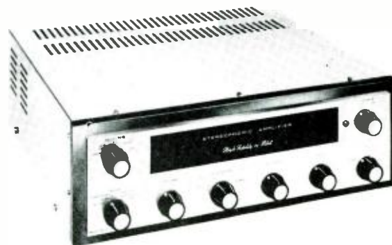
Fig. 8. Pilot SM-244 offers both preamplifier and power output for stereo use.
