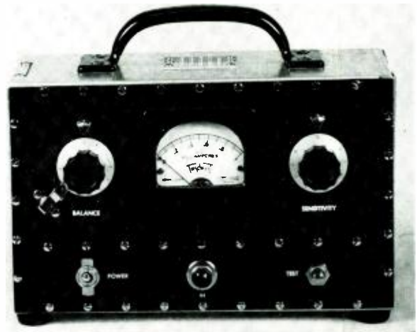
Fig. 9. Panel view of variable sensitivity tuning meter.
