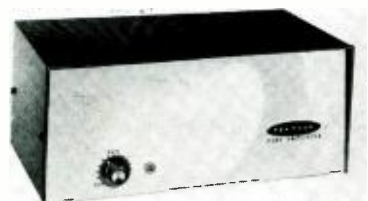
Fig. 5. Pentron CA-11 preamplifier—a single-channel playback unit.
