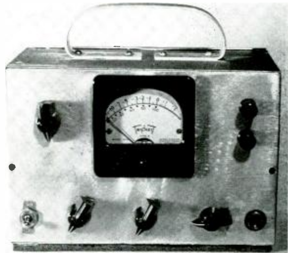
Fig. 1. Front view of remote amplifier. Note that phone jack is insulated from panel. Use of circuit-closing jack eliminates need for toggle switch shown.
