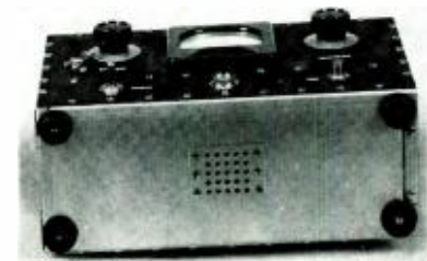
Fig. 10. Bottom view of meter, showing ventilating grille and rubber feet.
