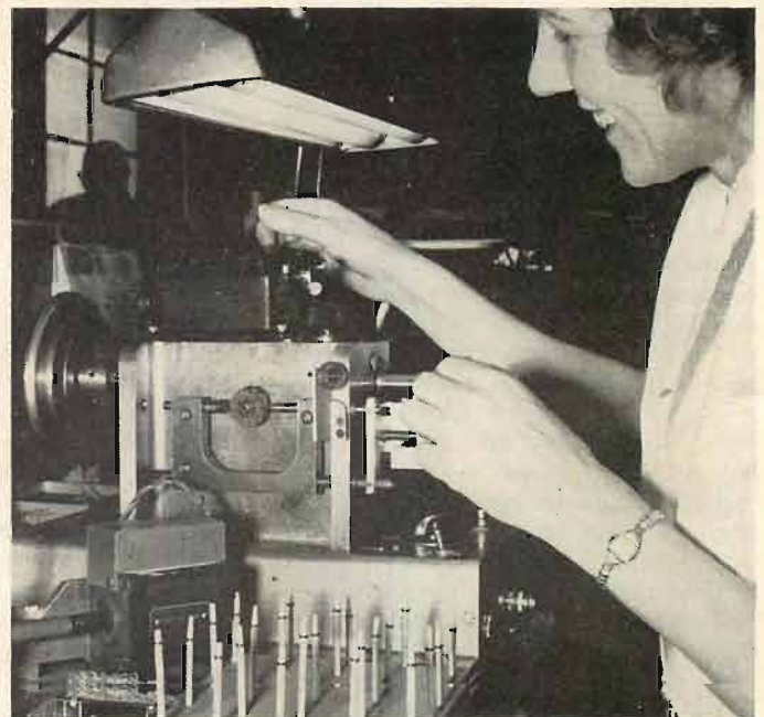
Fig. 6. Coil winding machine for pickup coils.
