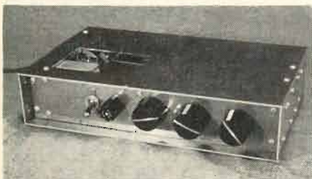
"Prettied up" model of the experimental translator. The third knob is an input attenuator.
