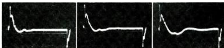
Fig. 6. Acoustic output of speaker, as monitored by microphone and oscilloscope, in response to step-front of low-frequency square wave: A (left), With amplifier damping factor of 6; B (center), with damping factor of 1; C (right), With damping factor of 0.1.
