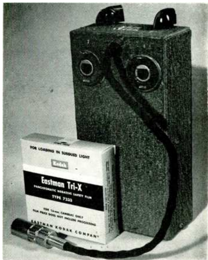
Fig. 1. External view of the two-channel sound-camera mixer unit—completely self contained, and suitable for employing two microphone inputs with a recording amplifier with only a single input.
