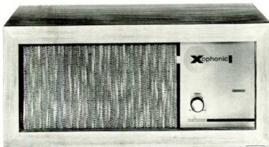
Fig. 6. Radio Craftsmen's "Xophonic," an artificial reverberation unit to increase the effective size of the listening room.
