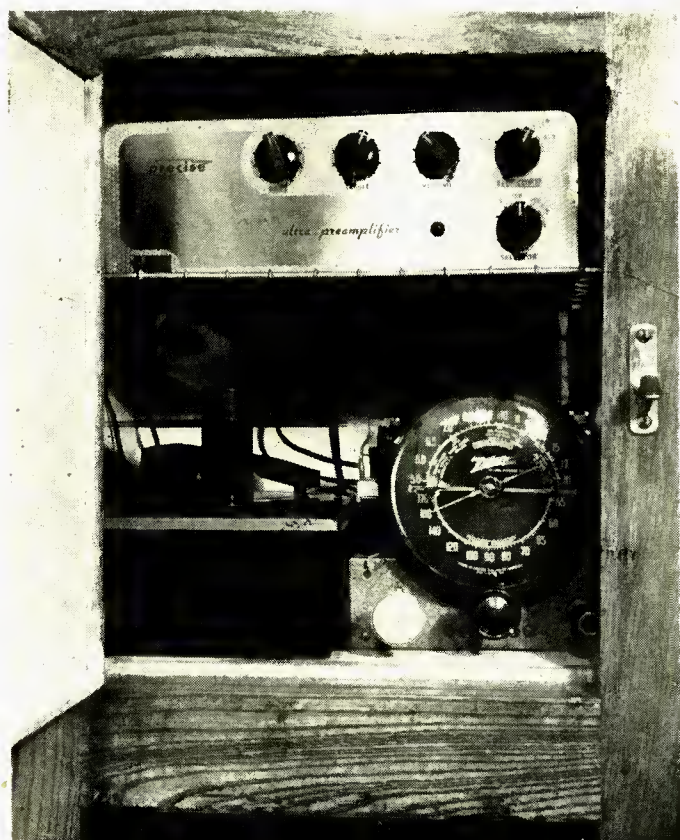
Fig. 3. Opening the door gives access to preamplifier, 45-rpm changer, and an old converted AM tuner.
