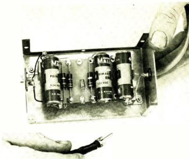
Fig. 3. Close-up of internal construction. Battery clips specified in parts list eliminate need for soldering batteries in place.
