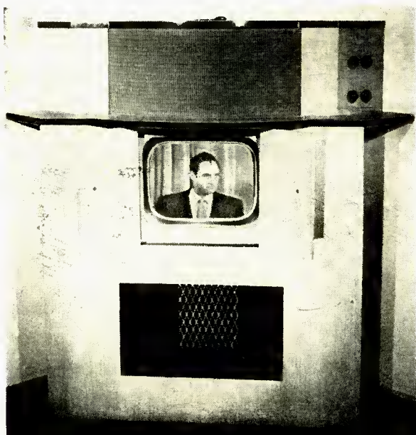
The two-way speaker system in a modern corner cabinet, with a 12-inch TV tube in the optimum location for the best illusion. Minor changes would permit the use of larger tubes, if desired, or its space could be occupied by the high-frequency speaker section, eliminating the superstructure.
