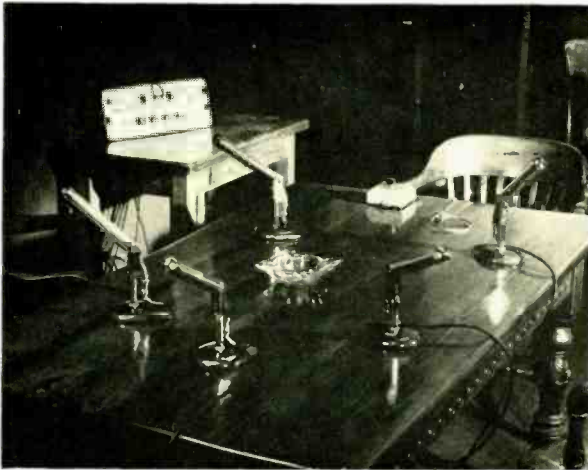
Fig. 2. The Conference Amplifier set up for use at a small meeting, with the five Electro-Voice microphones in typical locations.
