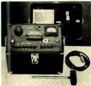
Fig. 14. General Radio Company's Vibration Meter is useful in isolating machinery noise.
