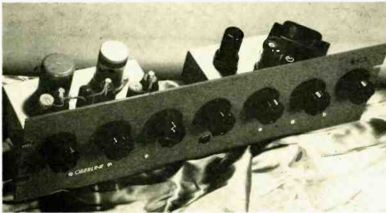
Fig. 2. Mixer amplifier with power supply on separate chassis (right) for minimum hum transfer to preamplifiers and input transformers. Note use of metal tubes and also that the power transformer is set at an angle. (Photo by Frank Aiello through courtesy of Oberline, Inc.)
