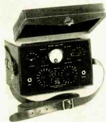
Fig. 11. Scott Sound Analyzer uses half-octave band pass widths.
