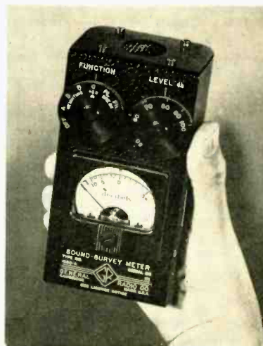
Fig. 3. Versatile pocket-size sound level meter made by General Radio.
