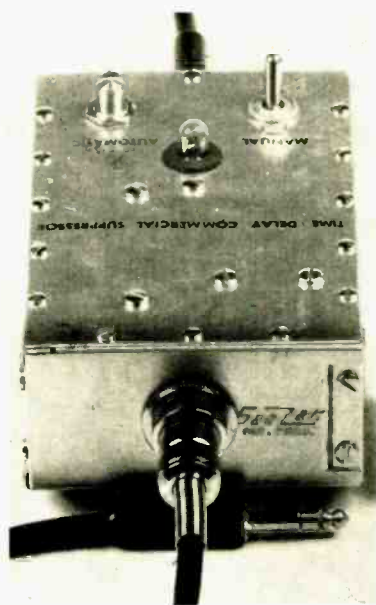
Fig. 5. Rear view of suppressor chassis shows use of Amphenol plug for connection from amplifier.
