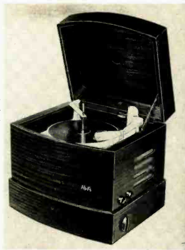
Fig. 4. The plinth below the Pye "Black Box" record reproducer incorporates an 8-valve pre-set three-station FM tuner controlled by plug-in quartz crystals.
