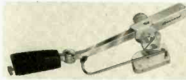
Fig. 5. The Garrard PA-10 transcription pickup arm is arranged so that the angle of the pickup head can be set to give the minimum tracking error and the vertical movement can be oil damped if required.
