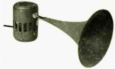
Fig. 2. The Ionophone D-15 loudspeaker made in England by Plessey. The unit shown contains the r.f. oscillator and the speaker "mechanism" itself which has no moving parts.
