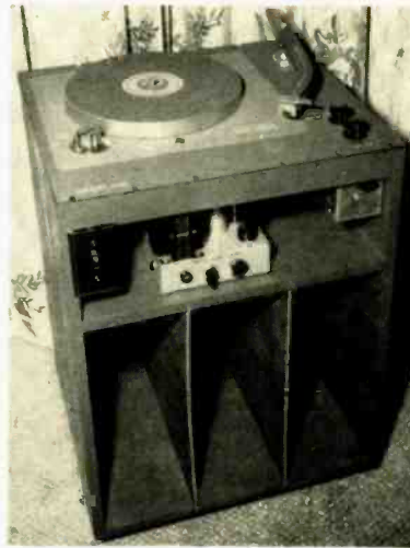
Fig. 2. Broadcast type turntable with equalizer and cueing facilities on pedestal. Mercury switch eliminates "popping" on motor starts and stops.
