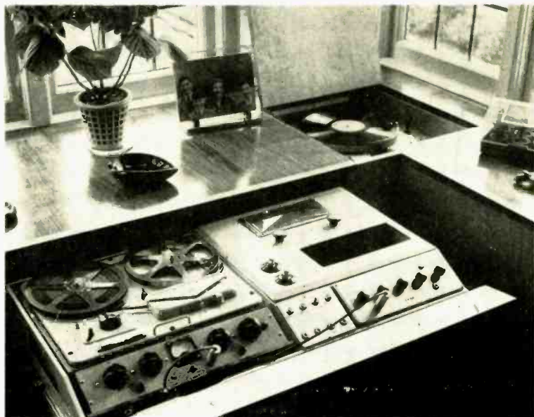
Close-up of the steel drawer in which are contained the tape recorder, amplifiers, tuner unit, crossover network, and a felt-lined recess for a microphone. On the right can be seen the transcription turntable and pickup.
