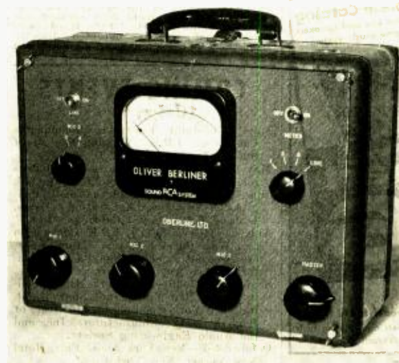
Fig. 6. Program line mixer-amplifier to drive tape recorder at proper level and impedance. Volume metering is also provided in addition to three microphone inputs.
