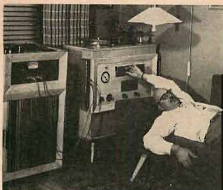
Fig. 7. Relaxing executive lies down to job of enjoying multi-source hi-fi system arranged for "automation." From the prone, preamplifier controls are within reach overhead; three switches in frame of couch are at finger's end of other hand for activating or muting tape recorder. Also shown are two cord sets in position at all times, from tape recorder output on preamplifier to input of tape recorder, through patch system, for recording. The other cord set goes from output of tape recorder to input of preamplifier for playback.
