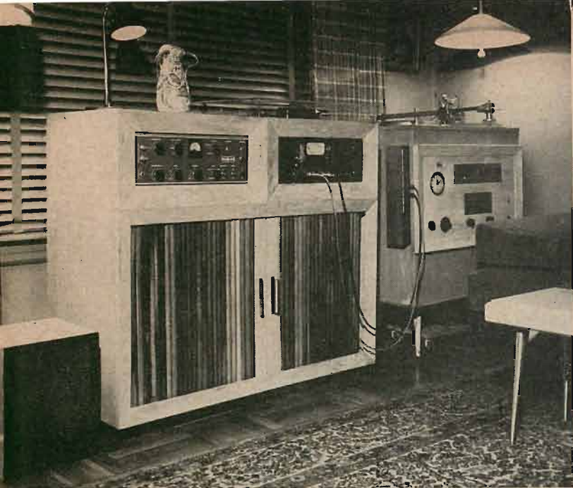
Fig. 1 (left). Setup of versatile hi-fi audio system along window-wall of 14 by 19 living room shows center cabinet housing recording amplifier and tape recorder; second cabinet houses record turntable and recording head, preamplifier, tuner, automatic clock, jack panel for patch system. Small cabinet lower left contains auxiliary speaker system, used also for monitoring recording amplifier in addition to headphones. Fig. 3 (right). Closeup of patch system strip showing insertion of hi-lo filter between pickup arm cartridge and preamplifier input. Clock is peg-controlled for presetting listening, recording or playback functions. Each peg represents 15-minute interval, providing precise programming and scheduling. Toggle switch over clock kills entire system.
