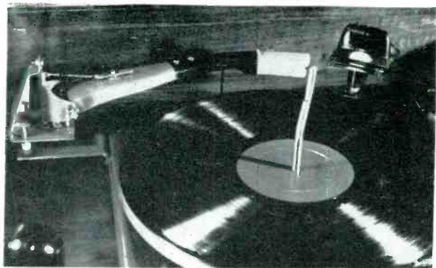
With a few simple modifications, an ordinary record changer can be improved to compare with hi-fi types with lowered record and stylus wear and reduced rumble. See page 21.
