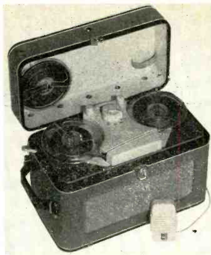
The Philips tape recorder, weighing only 21 lbs., incorporates a microphone, two reels of tape, and one empty reel. Single knob control operates through seven positions, and separate gain controls are provided for recording and reproducing.
