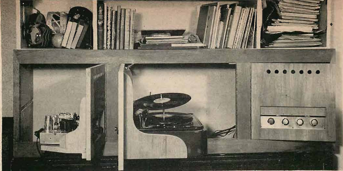
Fig. 10. The summing up: The bookshelf houses the components in depth; the walnut-veneer frame with doors does the load-bearing. Note flush setting of control knobs; also friction drop-lid hinge holding record player firm for loading and starting. Also that amplifier controls at the right are convenient to the player. Framework is secured to bookshelf with screws through the top rail. Material for frame is solid walnut, inside and out; doors, walnut-veneer.
