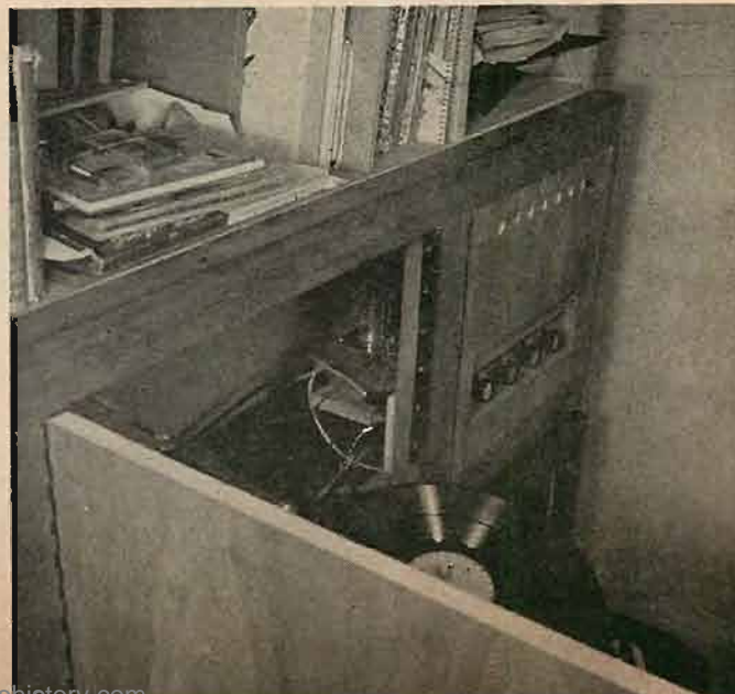
Fig. 6. Record player and amplifier-preamp are paired off for conveniently joint operation. With player door opened, amplifier inputs and level controls are easily right-handly. Note accessory 3-way plug attached to inner face of upright, powered from outlet in amplifier, and providing convenient, uncluttered hook-ins for tuner and record player power cords.
