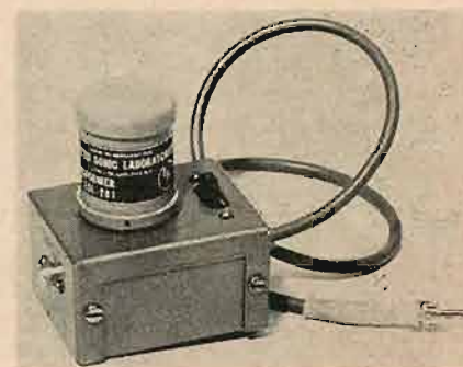
Fig. 4 (left). Top view of ESL Concert Series cartridge. The Standard Series is identical in appearance. Fig. 5 (center). Bottom view of Concert pickup showing stylus assembly. Fig. 6 (right). Transformer used with the ESL pickups mounted on a small chassis for instant plug-in use.
