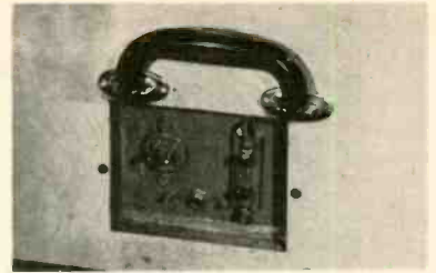
Fig. 5. Utility plate, located on the back of the cabinet, provides fuse mounting, a.c. inlet plug, and jack for tuner or tape recorder.
