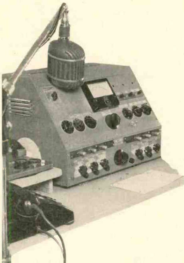
Fig. 1. The completed console in its operating position with the announcer's microphone directly above it.
