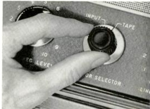
The Ampex 600 monitor selector switch lets you make an instantaneous listening comparison between what is fed to the tape and what the tape plays back to you. (Ask your local Ampex distributor for this demonstration*)
