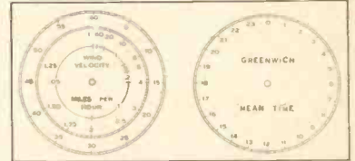
Fig. 6. Special timer scales made by combining standard drafting and trans-adhesive lettering.
