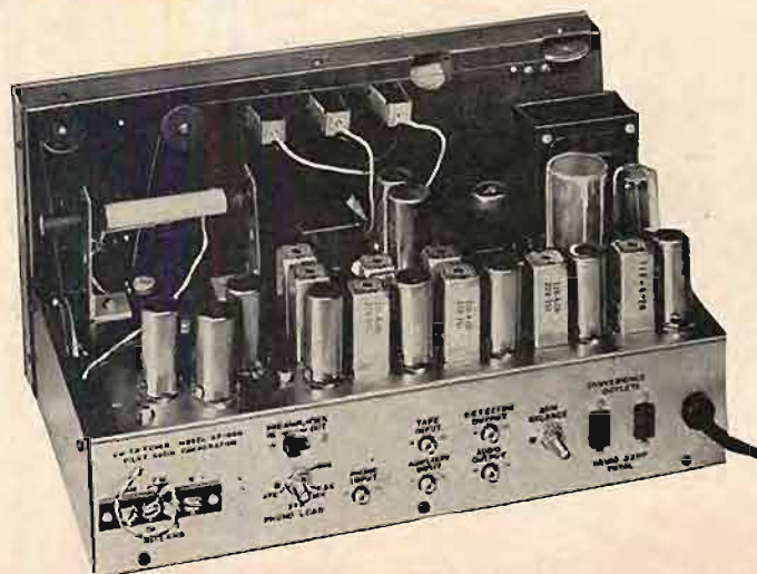
Fig. 10. View of AF-860 to show input jacks and rear apron controls.
