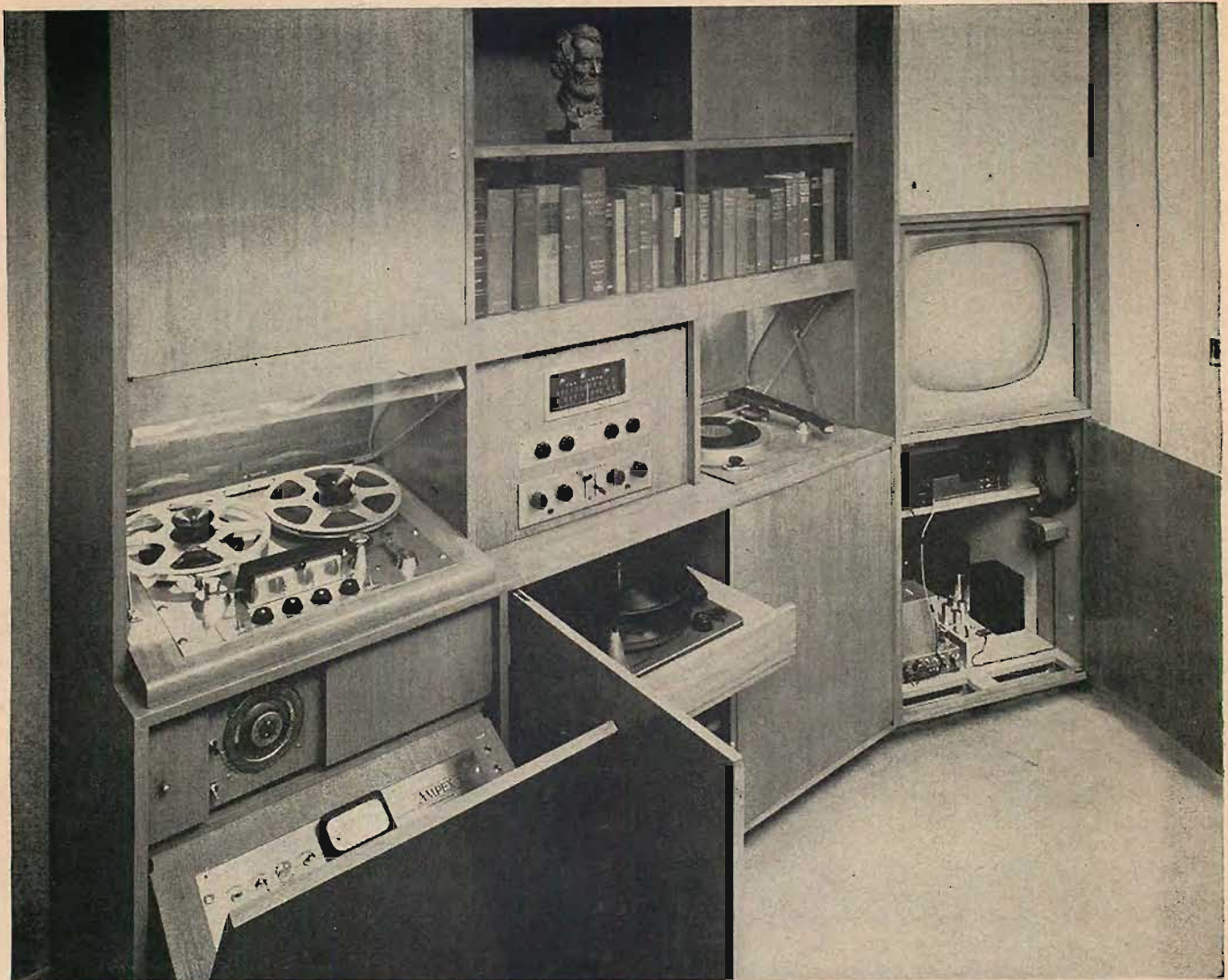
Fig. 3. Audio equipment grouped for convenient manual operation, also works completely automatically. Note 24-hour program timer below tape reel plate and controlling toggle switches alongside. Amplifiers feeding main and extension speaker systems are housed below 24-inch picture tube; also relay chassis and separate amplifier for TV sound. Main speaker system is behind screen over picture tube. Tuner and preamp are placed between tape recorder and turntable, with record changer on slide-out below.
