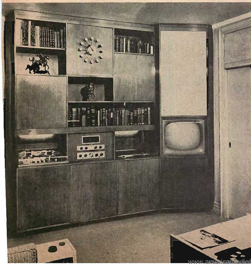
Fig. 1. Music wall takes a modest nine-foot square corner in room 12 by 18 feet, houses compactly a complex of hi-fi equipment, including professional tape recorder. Finish is sandalwood on mahogany-faced plywood. Clock at top is independent of audio system. Note Plexiglass hoods over tape reels and turntable. Remote TV tuner is in magazine rack.
