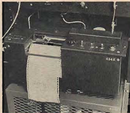
Fig. 5. The recorder automatically records frequency response on a calibrated chart. The recording pen is servo-driven.
