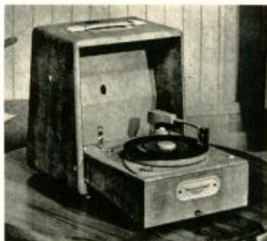
An all-wave 3-speed radiogram—H.M.V.'s Model 1507—one of the most compact and lightest units of its type ever made.
