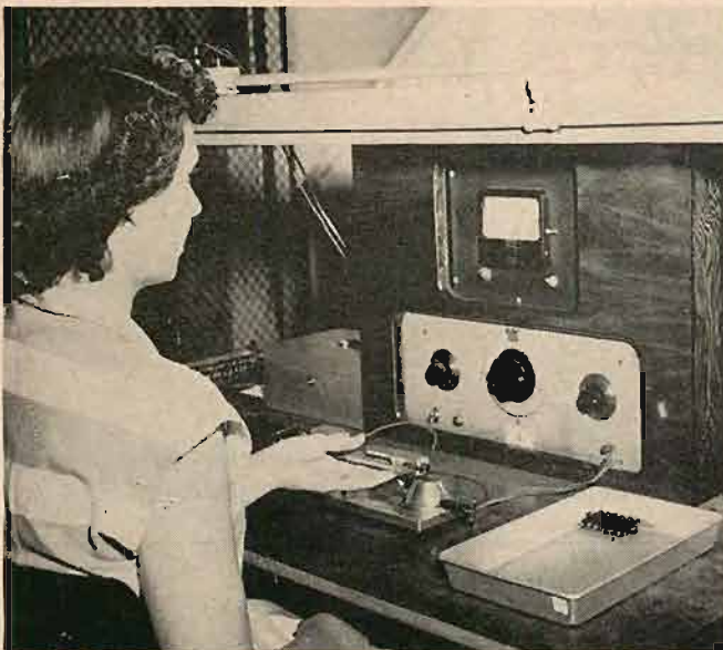
(Left) Production testing of compliance, using a magnetically driven vibrating reed which is loaded by the stiffness of the cartridge. The change in amplitude of vibration is read from the meter which is calibrated directly in compliance—the reciprocal of stiffness. A high value of compliance is necessary to prevent distortion and actual damage to the record groove. (Right) Production testing of output voltage and frequency response. Voltage output at 1000 cps is indicated on the meter while playing a test record, and frequency response is checked within a 2.5 db envelope on the face of the oscilloscope over the range from 50 to 10,000 cps. The source for this test is a sweep-frequency record.
