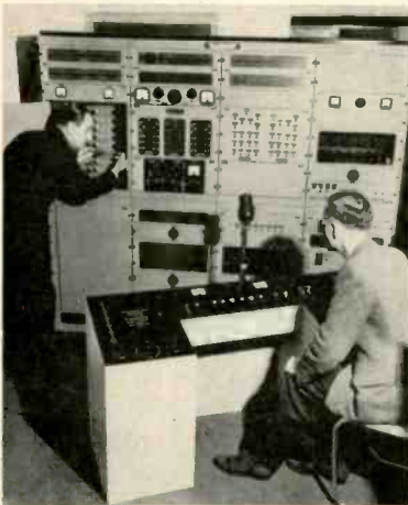
Fig. 1. Control panel and main equipment of Tannoy low-level sound reinforcement system in Canadian House of Commons.
