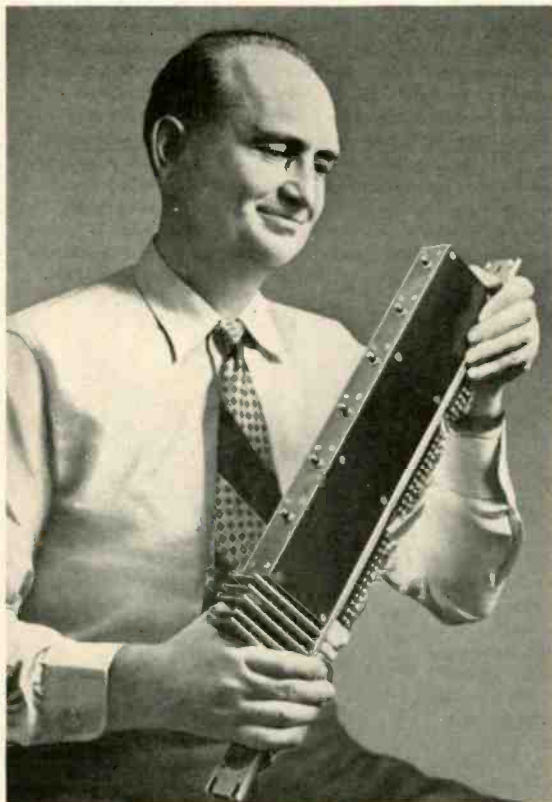
Laboratories engineer examines Transistor oscillator. It is used in Englewood, New Jersey, where 10,000 subscribers can personally dial distant cities. Transistors generate the signals which carry the dialed numbers to other towns and cities. Other uses are in prospect.
