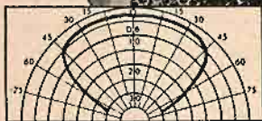
Directional characteristics of the acoustical lens at 5000 cycles.
