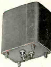
Miniaturized filter case is 1 11/16" x 13/16" x 1 1/8" height. Weight — .3 lbs.
