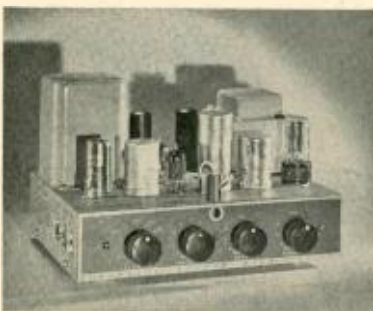
Fig. 4. The self-contained 10-watt amplifier.
