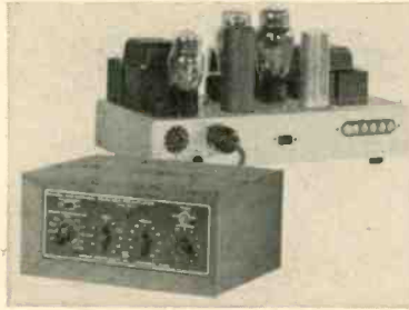
The Scott 214A amplifier, with remote control, which permits more convenient mounting in usual home cabinets.
