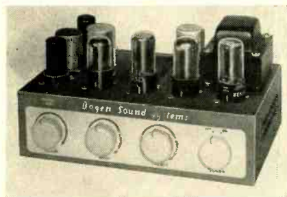
Fig. 4. Bogen DB-10 amplifier, typical of the smaller units used in unit-type systems.
