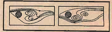
Fig. 4-3. Successive eddies formed by water flowing past an obstacle. (After Sir James Jeans, "Science and Music," The Macmillan Co., 1937.)
