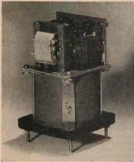
Fig. 9. Production model of 400-cps, 10-watt control amplifier—approximately same size as that required for a 5-watt audio unit. For audio use a different core material and higher-frequency carrier would be used. Photograph courtesy Magnetic Amplifiers, Inc.
