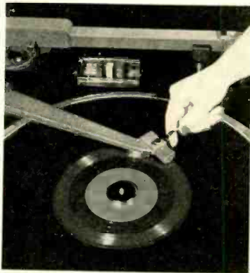
Fig. 1. New pickup and arm designed for playing both fine- and standard-groove records in broadcast station use.
