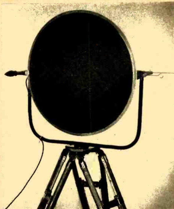
Fig. 4. Rear detail view of the parabolic microphone.
