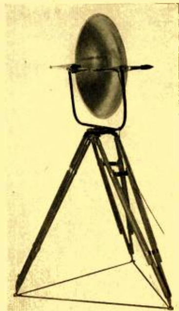
Fig. 2. The complete parabolic microphone unit mounted on a tripod.
