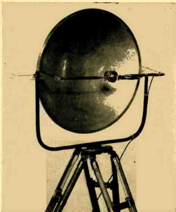
Fig. 3. Front detail view of the parabolic microphone.
