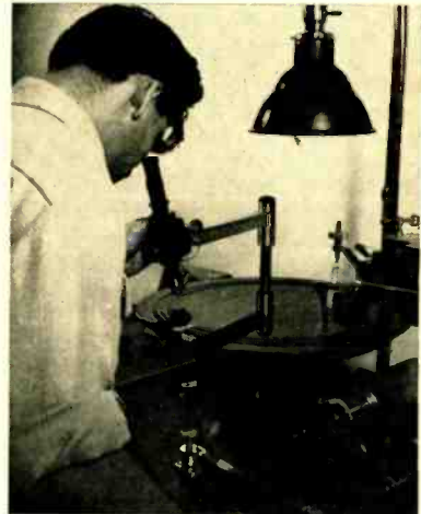
Technician checks grooves on transcription being cut on Scully lathe in Recording Section.
