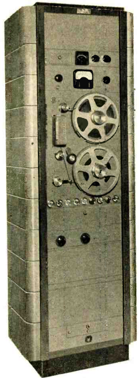
Fig. 1. Complete rack-mounted recorder for typical installation in a broadcast station or recording studio.
