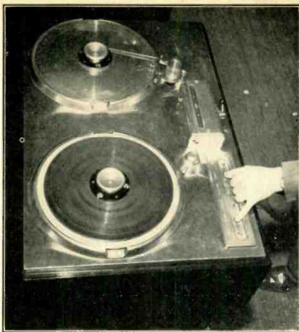
Fig. 1 (left). Top view of professional-type recorder (Ampex). The tape feeds from the loaded supply reel at the left past a tape guide which automatically actuates a motor switch. The control panel is shown below the supply reel, with the magnetic head assembly to its right. The drive capstan and pressure roller are at the right of the head assembly, with the take-up reel above. Fig. 2 (right). Motors and brake-drum assembly of the same machine.
