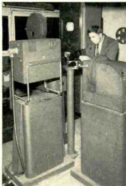
Fig. 4. The author adjusting a slide projector in the projection room. The film camera is at the left, 16-mm projector at the right, and the upper magazine of the 35-mm projector is visible above the film camera.
