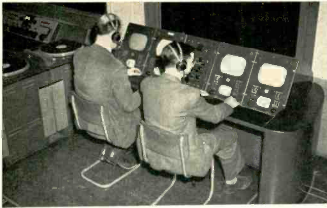
Fig. 2 (right). Small studio containing lights, microphone boom, and Image Orthicon camera. Fig. 3 (above). Video console with camera controls, "Studio B" switching, and master switching preview monitor.
