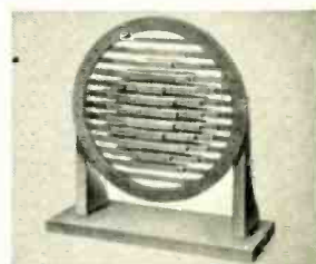
Laboratory model of the new lens. A similar arrangement of metal strips is concealed in the foam plastic blocks in the large picture.
