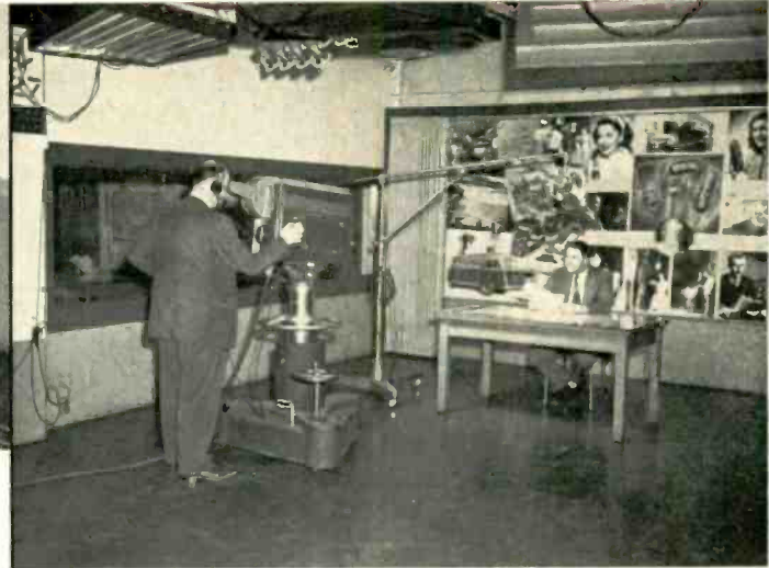
Fig. 2 (right). Small studio containing lights, microphone boom, and Image Orthicon camera. Fig. 3 (above). Video console with camera controls, "Studio B" switching, and master switching preview monitor.
