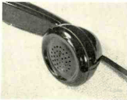
Fig. 2. The holes in this telephone mouthpiece have air resistance and mass which must be included in the design of the handset microphone.
