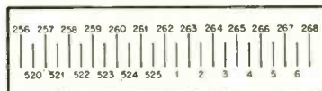
Fig. 2. Scanning lines of the TV picture during the "splice" caused by the shutter movement.
