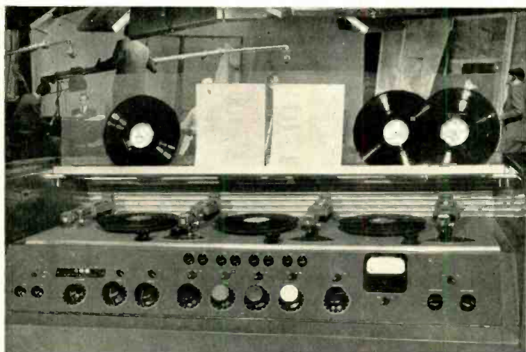
Fig. 1. A close-up of the operating controls of the CBS 4-A sound effects console. Immediately below the clear plastic script and record rack is the turntable platform upon which is mounted the three variable-speed turntables and four transcription arms. Lever arms controlling the turntable speed are to the right and forward of each turntable.
