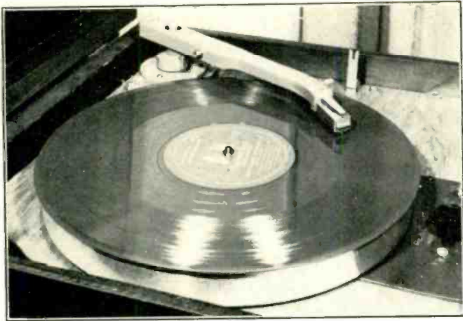
Fig. 2. Turntable and pickup assembly used with the control unit.
