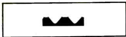
Fig. 3. Photograph of groove cross section showing "horns" thrown up on upper edges of groove.
