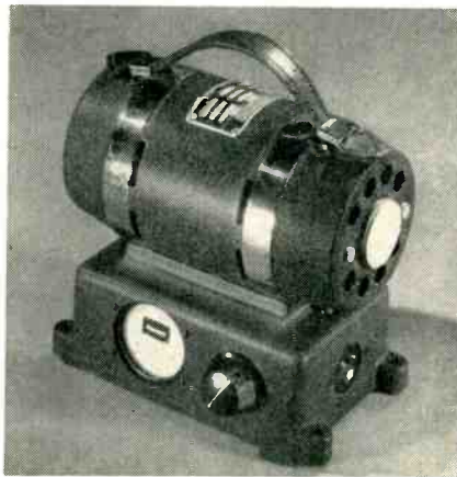
Fig. 1. Frequency Controlled Super Converter for broadcast service. Note rheostat control and frequency meter.
