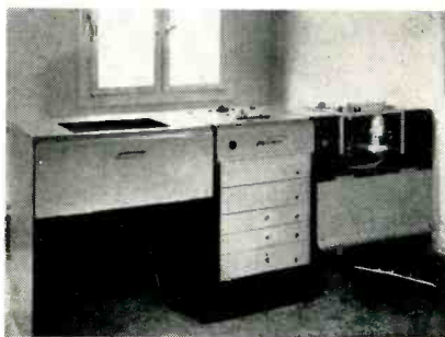
Fig. 2. Partially completed dual Magnetophon Unit. (Photograph by Wm. R. Busch, Chief Engineer for RIAS.)
