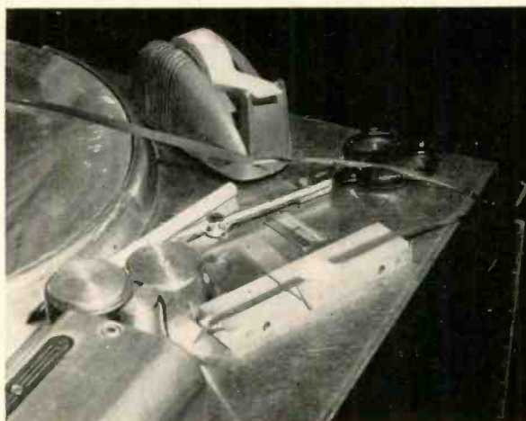
Fig. 5. Tape ends are joined together in the splicing block. The #41 Scotch tape is applied at an angle to the magnetic tape so there will be the least possible disturbance to smooth motion of the tape through the head assembly.
