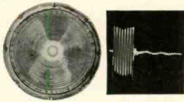
Fig. 11A (left). Cone breakup at 510 cps, with four radial nodes; point C. Fig. 11B (right). Transient response to same signal.
