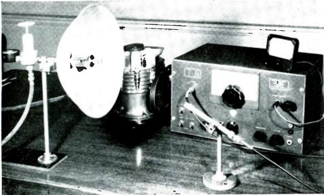
Testing Hartmann whistle in parabolic reflector.
