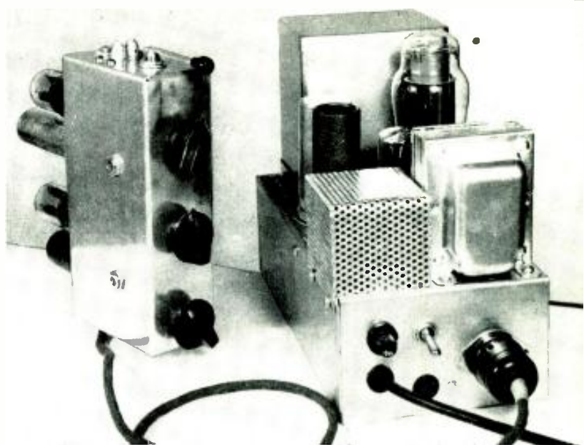
Fig. 1. Compact, two section amplifier with control section arranged for mounting in small panel area.
