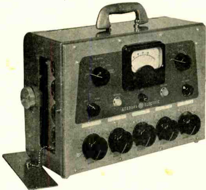
Fig. 1. Front panel of portable amplifier. Access plate at left end is removed to permit connection of microphone cables.
