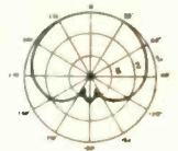
Tru-Cardioid pickup pattern. Wide angle pickup from the front, diminishing sharply to the rear with approximately 15 db discrimination between front and rear at all frequencies.
