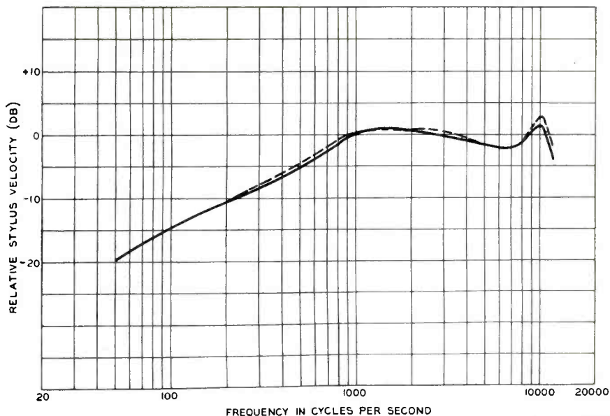
Fig. 4. Response measurements taken six months apart. Note only a slight change, an improvement resulting from controlled temperature operation.
