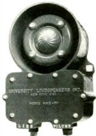
Fig. 6. Speech type horn loudspeaker designed for railroads, mines and hazardous locations. It has a throat diameter of 2½ inches, an air column length of only 8 inches, is characterized by wide dispersion angle.
