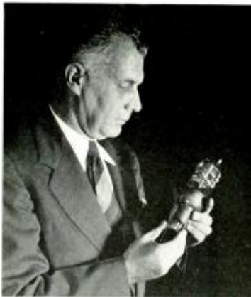
R. W. Sears of Bell Labs. holding a special tube which he developed for pulse code modulation transmission.
