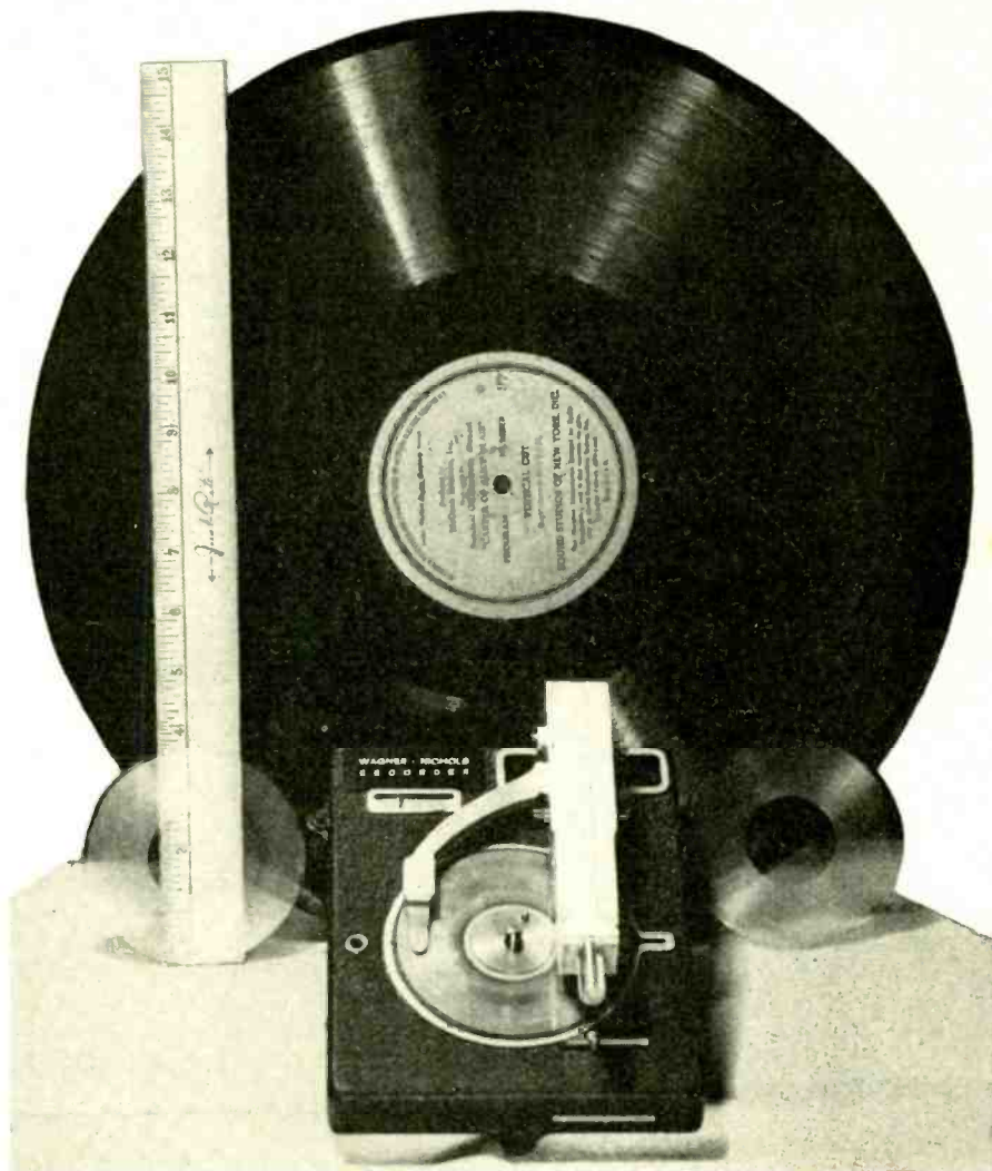
Fig. 1. The complete recorder unit is shown at the right. A 15-minute recording can be made on the small plastic discs shown. The arm and spring pressing on disc assure good contact between disc and tracking point following groove cut on back of blank.
