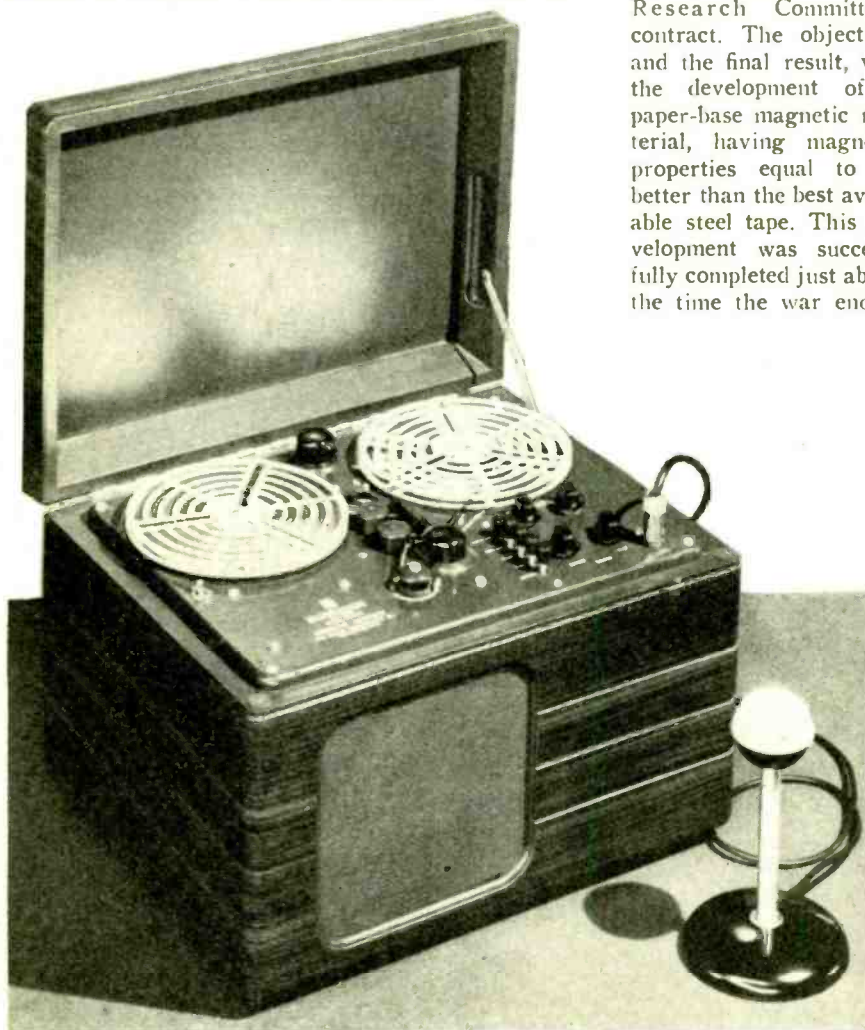
Fig. 2. The Brush BK-401 Soundmirror is a magnetic tape recorder having the general size and appearance of a conventional table-model phonograph. It is a complete recorder and reproducer and is capable of one-half hour of continuous operation. Recordings can be made from the microphone provided with the unit, from a radio receiver or any other source of audio signals. Convenient controls are provided to perform the various operations. The reels, which are 7 inches in diameter accommodate 1250 feet of 1/4 inch wide, paper-base magnetic tape.
