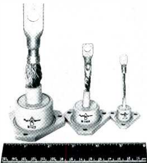
New high current silicon power rectifiers introduced by Audio Devices include models with 400 volt peak inverse rating, and maximum forward current ratings from 25 amperes to 200 amperes. Picture above shows extreme compactness of new rectifiers, which are hermetically sealed and individually tested at full load with temperature and humidity cycling. Unit on left shows size of 100, 150, and 200 ampere models; that in the middle shows size of 50 and 75 ampere models; and that on the right the 25 and 35 ampere models.
