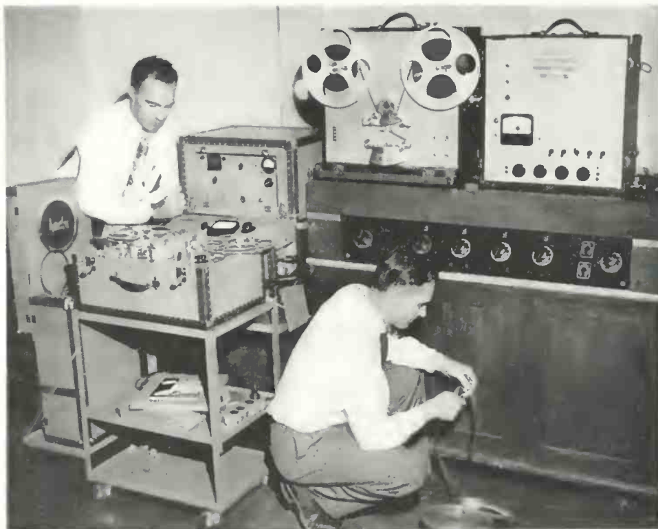
Engineers DeWitt Morris and Andrew Richardson, of Universal Recorders, checking a program on a Rangertone 1/4" tape recorder and Stancil-Hoffman 17 1/2 mm synchronous magnetic film recorder and reproducer.
