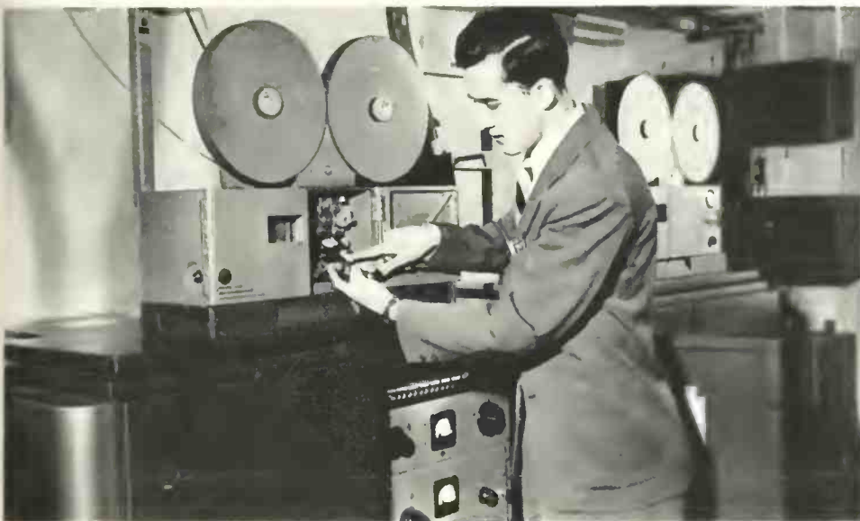
Fig. 6. Sound recording equipment at NBC television studios, New York, showing a pair of RCA sound on film recorders. Engineer Michael A. Maneale threads 16mm magnetic film into one of the machines. In this double system, sound is recorded separately from the picture, on both magnetic and photographic film.
