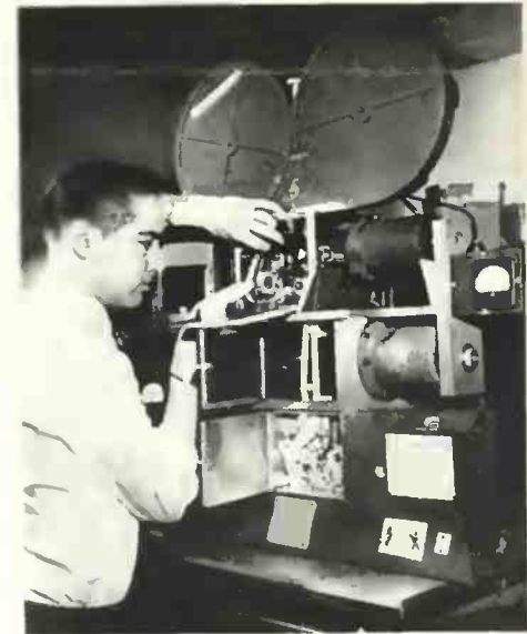
Fig. 4. Engineer Paul Ruckdeschel, of WJZ-TV, threads camera. Note wide separation between camera and optical sound recording unit below.
