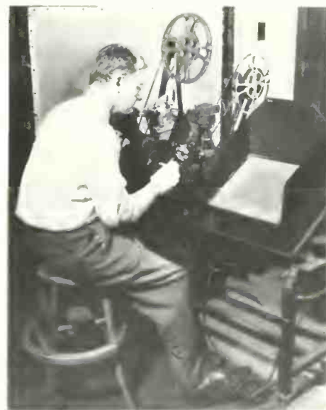
Fig. 8. R. M. Fraser, of NBC engineering laboratory, checks a recording on a modified Moviola editing machine, equipped with a magnetic head for playback of the 16mm magnetic film (at left). Picture print is on right hand reel.
