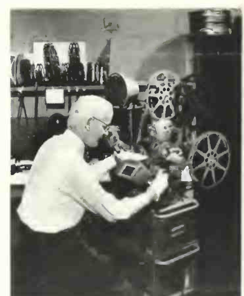
Fig. 5. Engineer Edward J. Greene demonstrates operation of Moviola sound film editing equipment, in one of the WJZ-TV editing rooms. Film at left is used for sound track, and at right, for picture. Any parts to be removed are marked on both picture and sound track, to be cut and spliced later.
