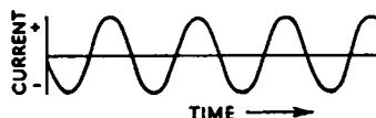
FIG. 1.4. A sounding tuning fork held in front of a microphone will give rise to a current waveform, as illustrated, of frequency coinciding with that of the fork.
