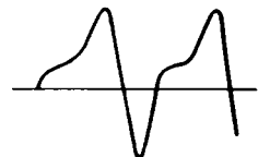
(Left) FIG. 4.7. Third-harmonic distortion. (Right) FIG. 4.8. Severe harmonic distortion caused by iron saturation in an output transformer due to an overload.
