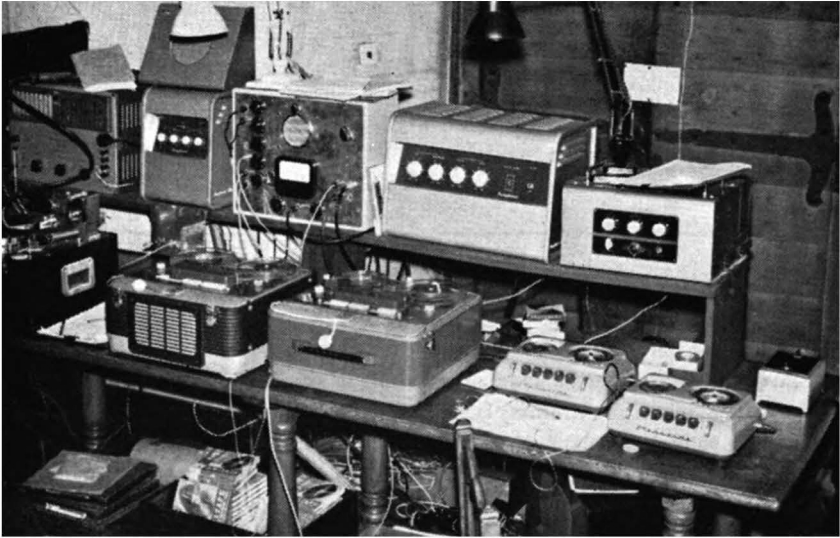
FIG. 9.15. Tape recorders and sound equipment installed for use at the Duke of Edinburgh's Study Conference at Rhodes House, Oxford (1956).
