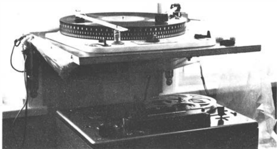
Fig. 9:1. One way of avoiding transmission of vibrations to the turntable is to mount it on the wall. A main structural wall should be used rather than a partition.
