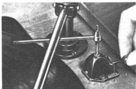
Pickup lifting and lowering devices are very useful. The Auriol Control and Decca Microlift are shown here.
