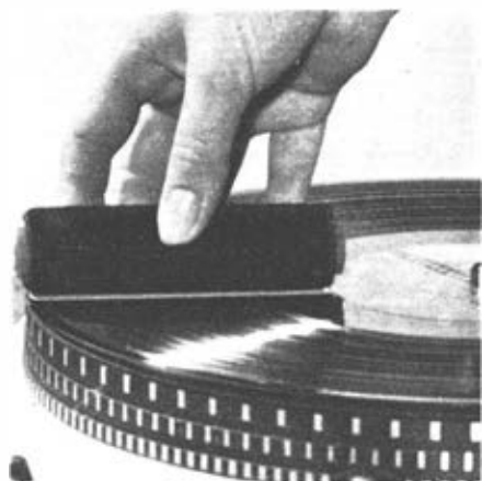
Fig. 5:10 (left) shows the Domestic Parastat , useful for thorough disc maintenance, while on the right (fig. 5:11) is the Watts Preener for removing superficial dirt.
